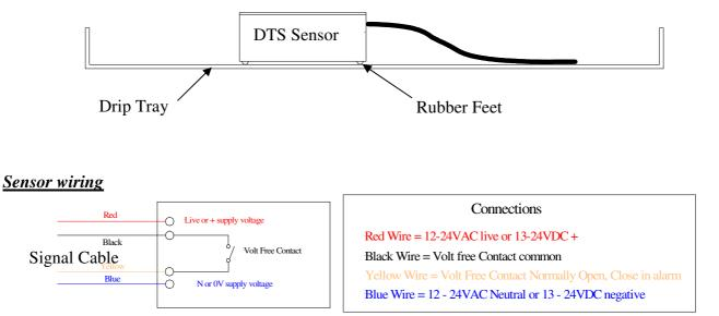
The signal cable should be terminated between the sensor and the main Alarm/BMS in the following manner.
