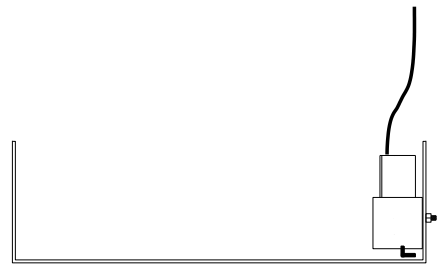
Deep drip tray side mounted using bracket (Sensor not to touch a conductive drip tray)
