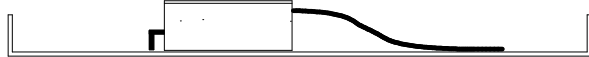
Drip tray without the mounting bracket (Sensor not to touch a conductive drip tray)
