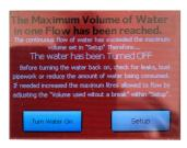
This screen will be displayed when the amount of water consumed within a single flow exceeds the alarm "Volume used without a Break" setting. Reasons for this alarm could be; a leak from a damaged fitting, bust pipework, fractured water tank, bath taps or garden hose left on.
