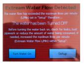
This screen will be displayed when the water flow exceeds the alarm "Current Water Flow L/Min" setting and could be an indication of a burst pipe. Another reason for this alarm to be activated could be that several kitchen appliances, sink, bath and garden hose are asking for water at the same time. If the unit is in automatic alarm setting update, pressing the "Turn Water On" button will automatically change the alarm setting to the to the new maximum.
