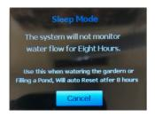
This feature is provided to allow long high-volume water flow periods to occur without tuning off the water supply. By pressing the "Sleep Mode" button, the system will stop looking at the water flow for eight hours or until the "Cancel button is pressed. Once the eight hours have elapsed, the system will automatically reset itself and start monitoring the water flow. This feature can be used when filling a fish pond or long periods of watering the garden.
