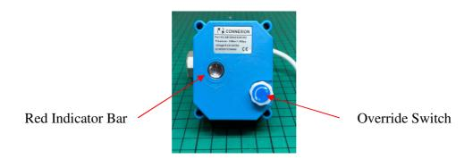
To take the valve out of shutdown and revert back to normal running, push the Override switch toward the blue housing allowing the valve to automatically open itself.
