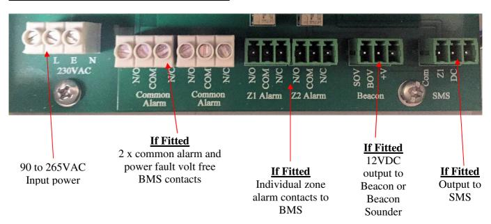
The Common alarm relay is normally energised, de-energised in alarm or power fault, therefore both "Common Alarm" contacts are identified correctly when the unit is powered and has no current alarms.
